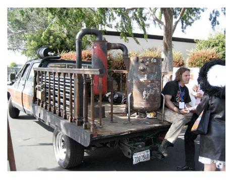
Figure 5: California Wood Burning Truck
