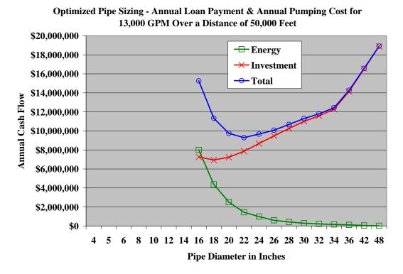
Graph 16. Optimized Pipe Diameter for 13,000 GPM and 50,000 Feet Distance
