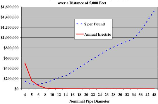
Annual Cost of Pipe & Annual Cost of Electricity for pumping 1,000 GPM over a Distance of 5,000 Feet
