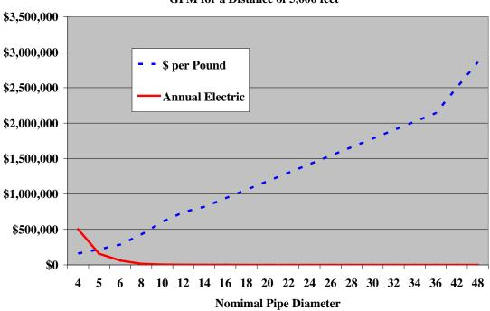
Pipe Capital Cost & Annual Electric Cost vs. Diameter for Flowing 1,000 GPM for a Distance of 5,000 feet
