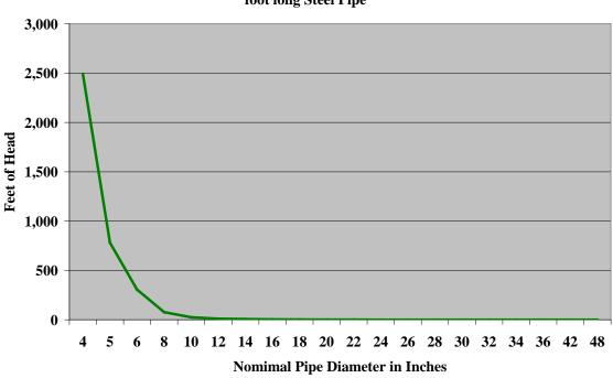
Head Loss in Feet of Water for 1,000 GPM of clean water flowing in a 5,000 foot long Steel Pipe
