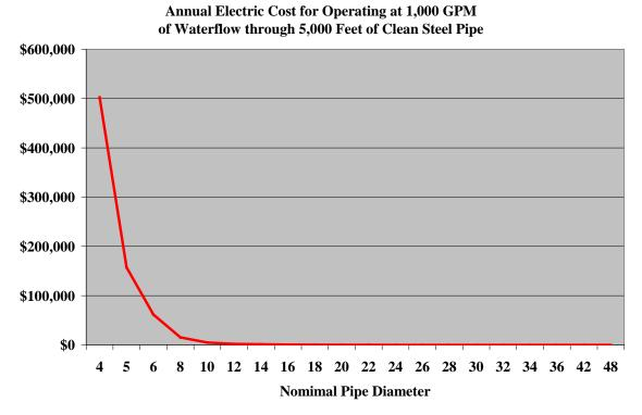
Graph 4. Annual Electricity Cost for Operating the Pump Motor
