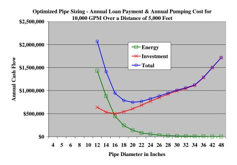
Graph 9. Optimized Pipe Pump Sizing for 10,000 GPM
